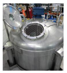
and reverse, effectively 'pulling' liquids off the floor of the vessel and distributing them evenly through the batch.
